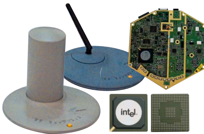
Airspan board (top right) using Intel's Rosedale chip, two views of which are pictured below it. To the left are two Airspan home modems using the board. The chunkier modem uses multiple aerials to boost range
